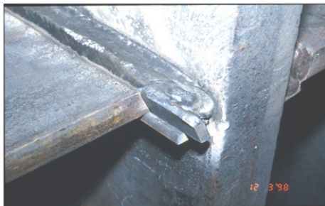
(a) Notch due to backup bar and weld tab
