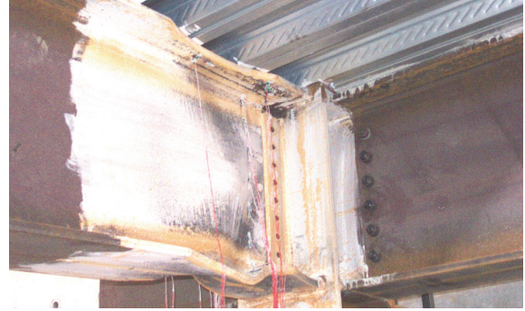
Fig. 15. Plastic hinge of DB700-C at 6% story drift
