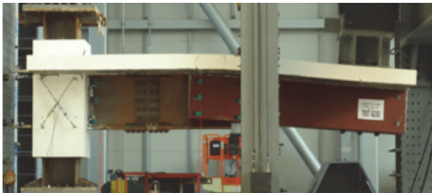
(a) W/O connection reinforcement; GC03
