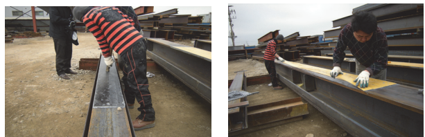
(b) Specimen fabrication procedure (CFRP/ AFRP)
