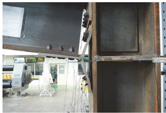
(b) Deformation of the G310-T15-B400 (Bottom T-stub)
