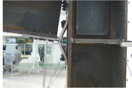
(b) Deformation of the G260-T15-B350 (Bottom T-stub)
