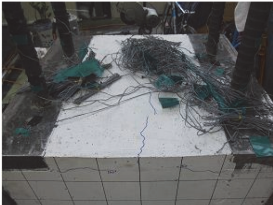
Fig. 15. Concrete crack of the improved form specimen
