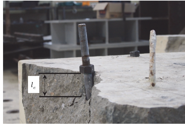
Fig. 14. Definition of bearing depth
