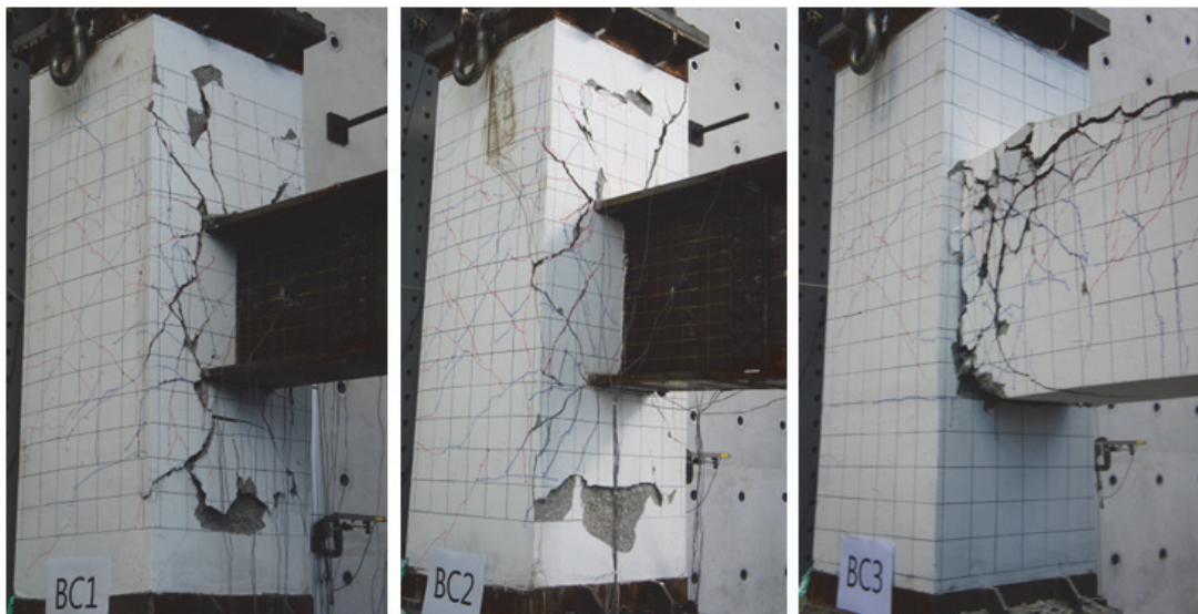
Fig. 9. Damage modes after the end of testing
