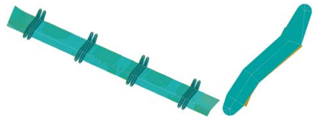
Fig. 13 Buckled mode shape of strut [6]
