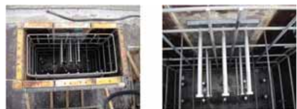
Fig. 11 Reinforcement and stud detail of specimens
