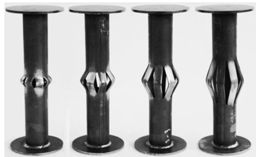
(b) S8 Type (From Left L=25, L=50, L=75, L=100)
