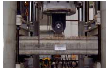
(b) Photo of pull-out test
