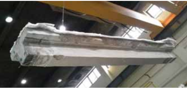
Fig. 8 Test result of spray-on fire protection
