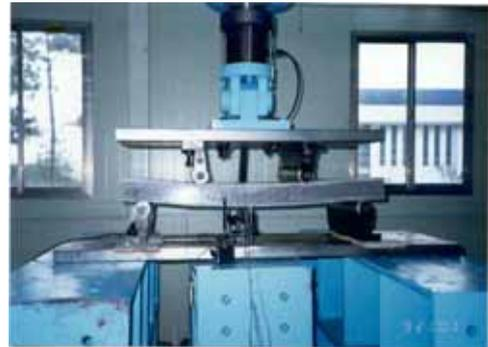
(a) Front view of 4-point bending test
