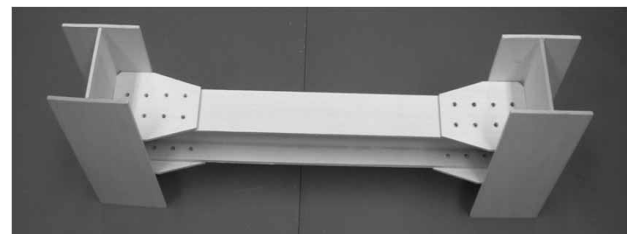
(c) Joining of the horizontal beams and the top welding plates using high-strength bolts and welding of the joints between the H-shaped steel columns and the top welding plates
