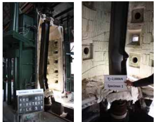
Fig. 3 The failure mode of test model B(S-1)
