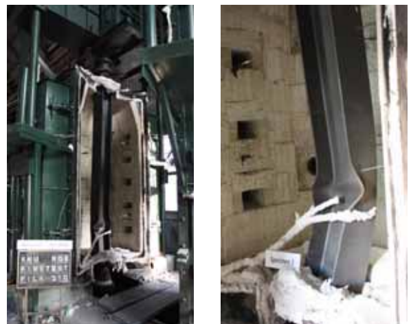
Fig. 4 The failure mode of test model C(S-3)
