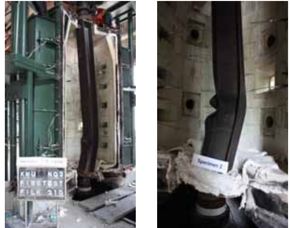
Fig. 2 The failure mode of test model A(S-2)
