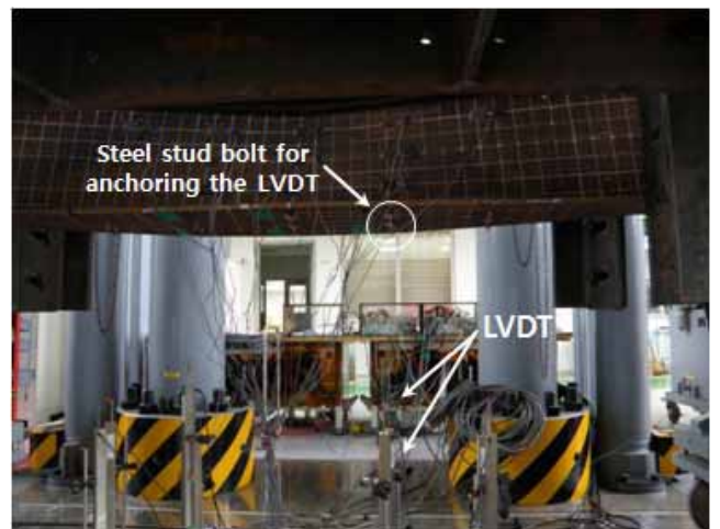
Fig. 9 Location of displacement and strain measurement instrument
