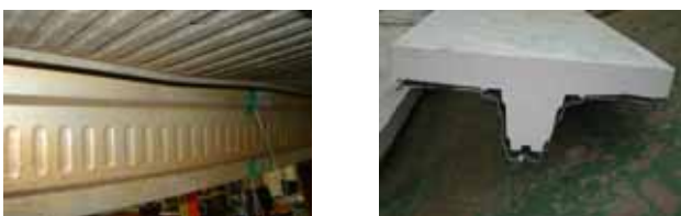
(a) Deck bending deformation (b) Bond failure Fig. 8 Fracture mode of specimens (SCS200-1.0R)
