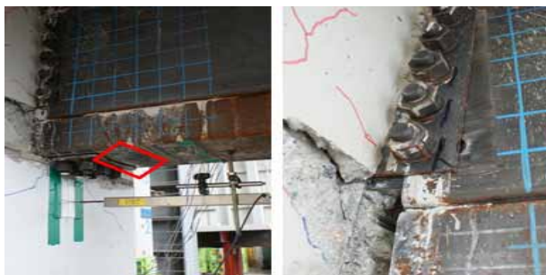
Fig. 13 Failure Shape of HF5-S-8 specimen : Local Buckling and Bearing Failure
