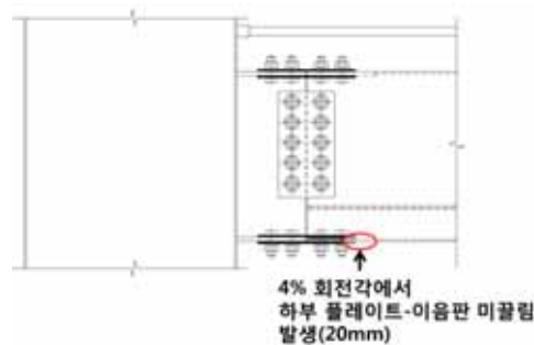
Fig. 16 Failure Shape of HF5-A-8 specimen
