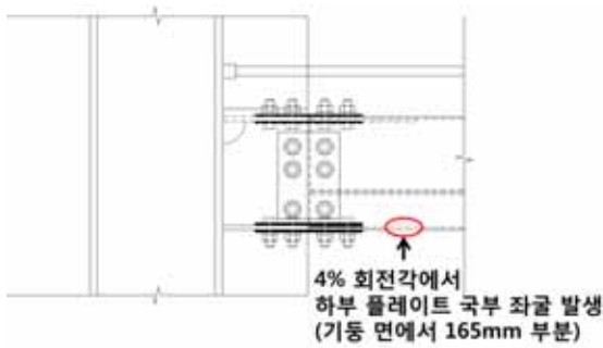
Fig. 8 Failure Shape of HF3-S-6 specimen
