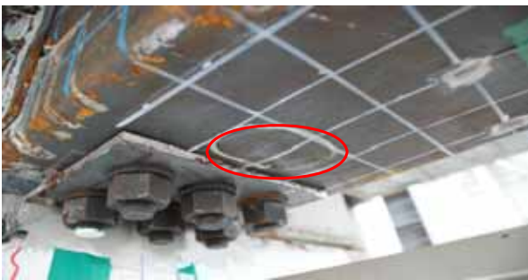
Fig. 9 Failure Shape of HF3-S-6 specimen : Local Buckling
