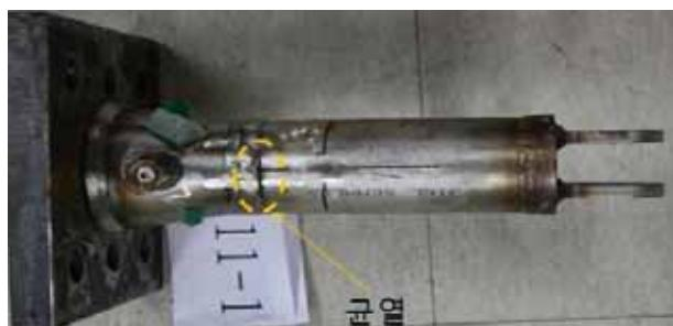
(a) Cracking from Weld Toe
