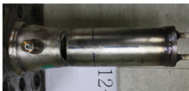
(b) Cracking from Initial Crack
