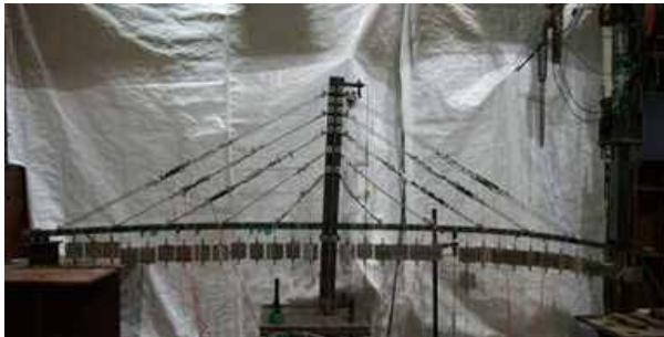
Fig. 25 Failure Mode of Semi-Harp Type
