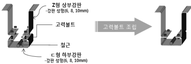
Fig. 1 Assembly of U-shape Composite Beam
