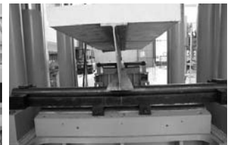
Fig. 16 Lateral buckling of H-composite beam
