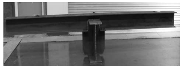
Fig. 4 Test Specimen of New Temporary Bridge system
